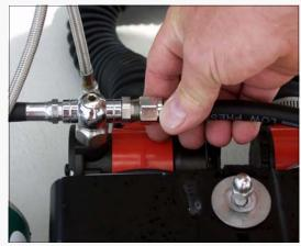
\*NOTE: The oxygen delivery system attaches to the rebreather via the elbow on the exhaust pod. Please note that the male end of the elbow which screws into the pod is NPT, or pipe thread. This is a tapered thread, NOT a straight thread. If you screw a fitting with a straight thread, such as a swivel elbow, into this port, it will damage the pod! If this happens, it is NOT repairable. Prior to modifying your rebreather, please be certain that you understand what fittings are required.
