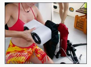
Rinse out the canister with fresh water to remove any old scrubber material. Once clean, disinfect the canister, lungs, breathing hoses and DSV if necessary. Ensure that the o-rings on the counterlungs and attachment areas of the canister are clean and free of debris and apply a small amount of lubricant. Re-attach the lungs to the scrubber canister. Remember to push them on straight and ensure that the o-ring is not pinched.
