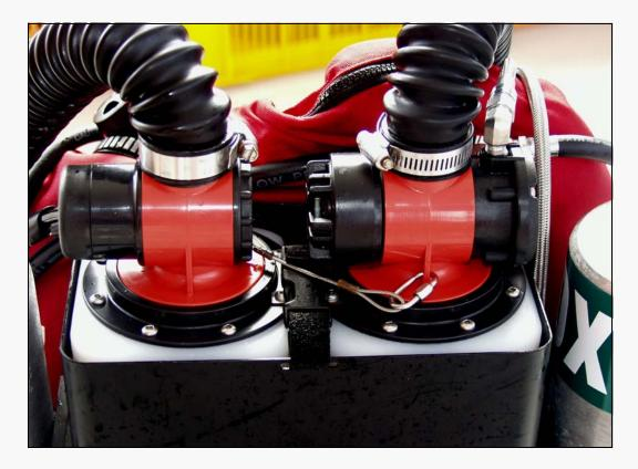
The scrubber canister holds five pounds of scrubber. It is a bi-axial design which allows the gas in the loop to pass through the scrubber two times. The KISS rebreathers were tested with Sofnolime 797 grade and this is what we recommend.
