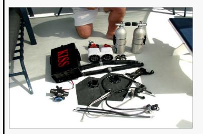
After verifying that you have all the necessary parts to assemble your new Sport KISS CCR, you are ready to put the pieces together. Start with the counterlungs and scrubber canister.
