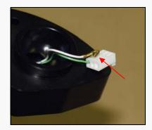
To remove the molex connector, push down on the two gold contacts as shown in the upper left photo. You will need to use a small tool such as a dental pick. Gently pull the wire out as you are pushing down. Take note on how the connector comes out of the contact. It will need to be attached in the same way. Also make a note on what position each wire is in. If you reattach the wires backwards, you will have a - sign in front of your digital PPO2 read out.
