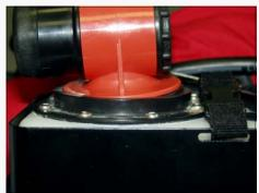
\*NOTE: Care should be taken so the bottom screens of the display & exhaust pods are not damaged. If the screens come off, the absorbent will be loose and can travel up the loop hose to the mouthpiece!
