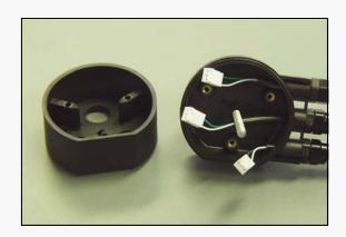
Next, remove the 3 screws. Note how secure the screws are as you remove them. There is no need to overtighten when you reassemble!!
