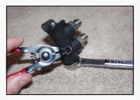
Remove the nut with either the wrench or alan key, depending on which nut you have; pull out the spring. The spool and orifice are all that is left inside the valve.
