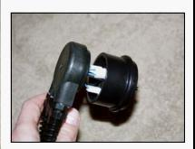
Plug the sensors into the white molex connectors. Once connected, check the displays to see if you are getting "negative gas". If you have a minus sign in front of the reading, you will need to turn the corresponding molex connector around. This will eliminate the minus sign. Unfortunately, there is no way to determine which is the correct way until you actually hook the connector up. Note that this will not effect the accuracy of the reading; it will just give you a minus sign in front of it.
