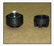
Once the valve is open, you will see a small white button sitting on top of the spring. Carefully remove the button and set it aside (remember which way it came out). Remove the spring and stretch it out a slight amount and then replace it. Re-insert the button, replace the top of the valve and tighten.
