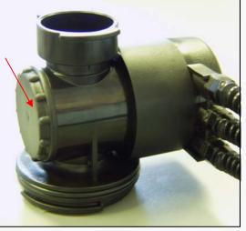
Once the knob has been removed, pull the sensor housing assembly free from the display pod.
