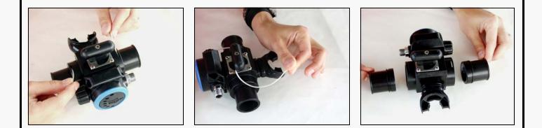
First, remove the monofilament by lifting it with a sharp dental pick and then pulling it out of the groove with a pair of pointed pliers or forceps. This will release the hose sleeve retainers.
