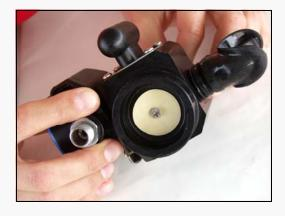
Once the monofilament is removed, pull the hose retainers out of the body and shake the valve plates loose.
