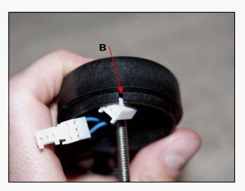
Push the sensor pod and the end cap with the molex plugs together. Note that the rib on the sensor pod, A, connects with the slot on the end cap, B.
