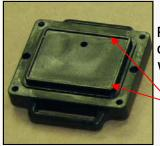
Replace the O-ring in the case. If you are reusing an O-ring, it will have kept its shape. It can go back into the case in the same orientation that it was in before. The lubricant will assist in keeping it in position.
