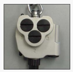
The VR Technology pendent display has 3 PPO2 readouts which read 3 individual sensors, an independent battery compartment, and 3 calibration potentiometers, one for each sensor. This is a great display for those who want a simpler system for battery changes and calibration. As the case is not opened during calibration there is less risk of flood damage. Also, the battery change is quick and simple as only one part needs to be undone. This makes any last minute battery changes simple and fast!
