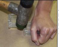
Apply lubricant to the puzzle pieces which join the displays together and then push the pieces together by hand. (ensure that you have them oriented the correct way). You should be able to push them about 1/8 to 1/4 inch together. Then, lay the cases on the table and gently tap with a rubber mallet until the edges on the back are even. Tap gently in the area where the cases join. See photo on the left.
