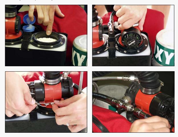
Once the hose attachments are back in place, re-attach the quick link safety tethers and the rubber LP hose.
