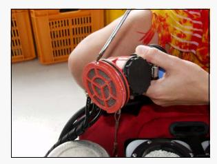
Chances are that a small amount of scrubber has collected in the edge of the hose attachments. Use a tool with a sharp end to clean out the debris. This will ensure a good seal and will make re-attachment easier.
