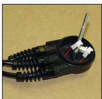
Once the wires have been secured to the connector, the other end can be attached to the display case. First, twist the wire counter clockwise 6 to 8 full revolutions. Then insert into the clear cover and tighten by hand. For the last 1/2 to full turn, use a wrench and tighten until seated. Twisting the wire prior will ensure a straight wire once you have finished reassembling the display case. Follow the directions on page 42 for reassembling the case properly.
