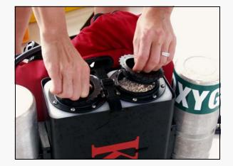
Attach the scrubber canister caps onto the top of the scrubber.
