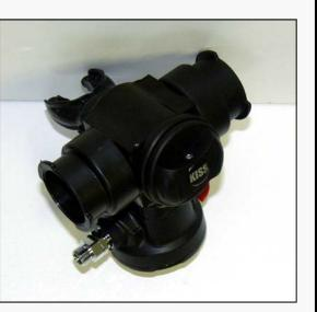
First the hose attachments should be removed. Do this by removing the U-clips, then pull the hose attachments away from the body.
