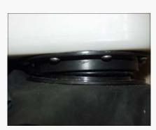
Lightly lubricate the o-ring on each counterlung and also the inside edge of the counterlung attachment on the bottom of the scrubber canister. Then attach the counterlungs. They are attached by pushing them onto the canister and doing a 1/4 turn clockwise. When correctly attached both lungs will be facing the same direction.
