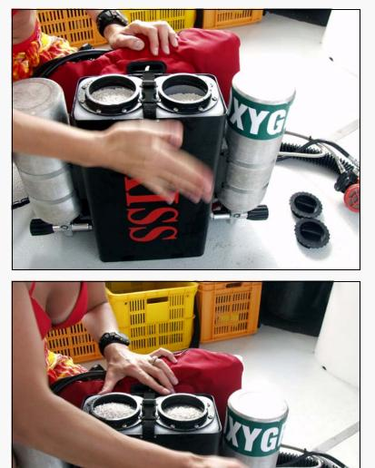
The final topping up of the container may require small amounts of scrubber being added along with slapping or shaking to settle it.
