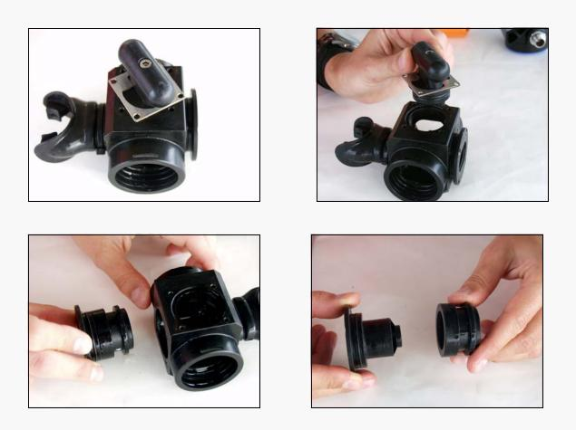
With the screws removed, turn the selector knob slightly counter-clockwise. This will cause the spool guide to pop out of position and protrude from the front of the body. Pull the knob out of the body. Once the knob has been removed, pull the spool guide and spool out of the body as well.
