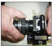
Finally to attach the breathing hoses to the DSV, push the hose stubs onto the DSV adapters, push down and turn right. Repeat to attach the other hose ends to the hose attachment pods.
