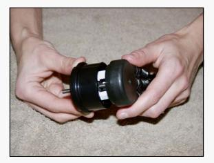
Once the molex connectors are attached correctly, push the sensor pod and end cap together, lining up the rib and slot so that they connect. Ensure that the wires are not pinched.
