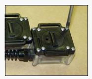
Take the display and with the calibration port side down gently tap the display on your thigh to remove any water droplets that could still be on the display back. GENTLY!! Even if you have been out of the water for some time, you should still do this.
