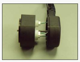
Attach the white molex connectors to the sensors, ensuring that they are pushed all the way in.
