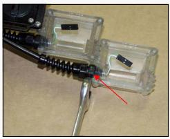
\*NOTE: Do not touch the other nut on the strain relief. This is used to attach the strain relief to the wire. Generally, a strain relief can only be used once. If you loosen it or remove it, it should be replaced. Also, it is normal for the 2 nuts to have a gap between them.
