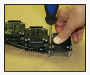
Place the screws in the holes and turn them slightly counter clockwise until you feel them drop into the old threads. Then tighten the screws until the back is secure and seated properly. While it is important that the screws are tight enough, it is also important that they are not over tightened. Remember, the O-ring creates the seal.
