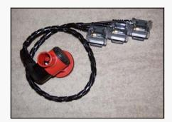
\*NOTE: The output for the K-ID sensors is 10 +/- 3 mvolts. This means that they should function accurately in a range of 7 to 13 mvolts. Also, always ensure that the sensors can be calibrated in air & pure oxygen. A volt meter can be purchased at any electronics or hardware store.
