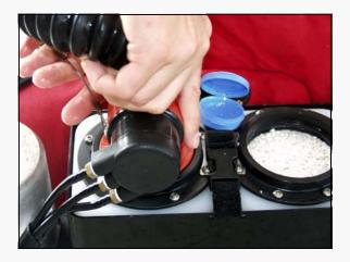
Lightly lubricate the o-ring on the hose attachments and the inside surface of the scrubber canister.
