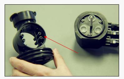
Once pushed together, attach the sensor knob to the opposite side and secure. Ensure that the knob is tight! The O-ring should be lubricated.
