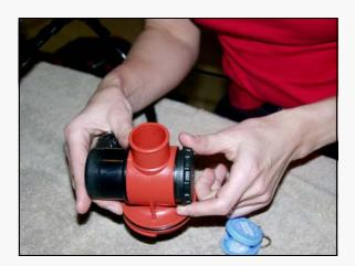
Lubricate the o-ring on the sensor pod and attach it to the hose attachment by screwing the end cap onto the opposite side. When screwing on the end cap, ensure that it is straight. Hand tighten until snug.
