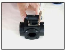
Once the regulator has been removed, remove the two screws on the spool guide and the four screws on the selector knob.
