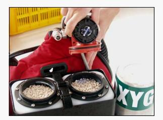
Remove the two hose attachments by rotating them 1/4 turn counter-clockwise and pulling up.
