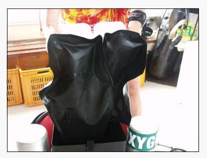
Once both counterlungs are attached to the canister and you have ensured that they are both secure and are facing the same direction, insert the canister back into the counterlung case. Remember, the bottom tips of the bags should point towards the BCD.
