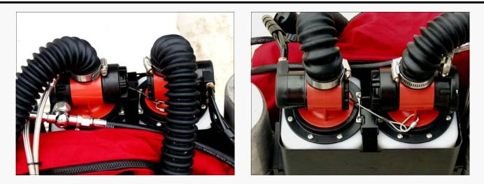
The next part to assemble are the hose attachment pods. Once complete, they should look like the above two photos. As this section is covering assembly, please see page 22 for proper scrubber filling instructions.
