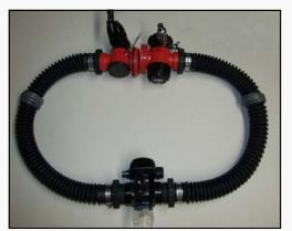
hose stub into position. Place the hose ring and hose clamp over the hose and hose stub, and secure. Repeat with the remaining 3 hose stubs. Once attached, pull on the hose stubs to ensure that they are securely fastened. A small amount of lubricant can be used to assist in pushing the hose stubs into position.
