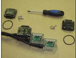
To change the clear display cover, start by following the directions on page 41. As well as having the display backs off on the case that you would like to change, the O-ring, wire and circuit board assembly must be removed.
