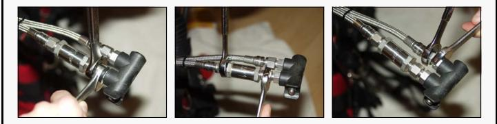
When attaching the value to the filter and the hoses, it is very important that you use a second wrench to hold the nut next to the value body in place. Do not allow this nut to spin as it will over-tighten and strip the plastic. This will cause the value to leak.
