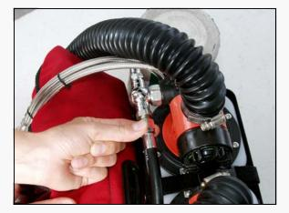
Changing the scrubber on the Sport KISS is quick and easy and takes just minutes. To start, unclip the two quick link tethers and remove the rubber LP hose which is connected to the inside of the T-connector swivel. The quick link/split ring tethers keep the pods from spinning and also hold the scrubber canister in place.
