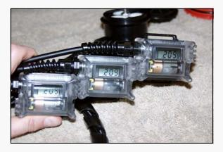
\*WARNING: After diving, gently tap the display on your thigh to remove any water trapped in the back of the display before opening the calibration port. A single drop of salt water on the electronic board or meter will ruin them!!! Gently means, do NOT use compressed air!!
