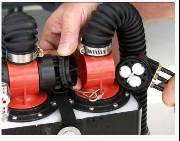
\*Warning: Ensure that the sensor housing & cap are tightly secured and that there is no gap showing, as in the photos above.
