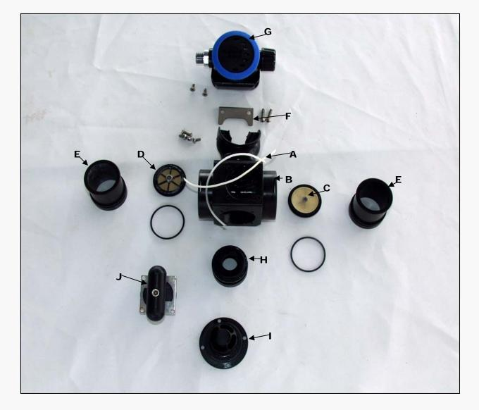
A: Monofilament B: Body C: Exhaust Valve Plate D: Inlet Valve Plate E: Hose Sleeve F: Regulator Attachment Plate G: Regulator H: Spool I: Spool Guide J: Selector Knob and Selector Knob Plate
