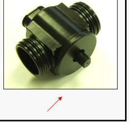
Now the inner barrel needs to be removed. it is difficult to pull out, push the switch onto the inner barrel stub, and then turn and pull. This method should easily allow the barrel to be pulled out.
