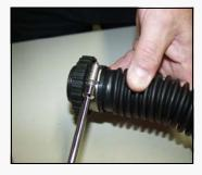
**\*WARNING:** IT IS IMPORTANT THAT ONLY A VERY SMALL AMOUNT OF LUBRICANT IS USED TO ATTACH THE HOSE STUBS. TOO MUCH AND THE HOSES WILL NOT STAY SECURELY ATTACHED TO EITHER THE HOSE ATTACHMENT PODS OR THE DSV.
