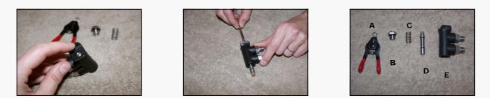
To remove the spool and orifice push in the button using a jewellers screwdriver. This will force the spool and orifice out the other end. When you have the spool removed, cut the old o-rings away with a sharp knife and replace them with new V75-008 o-rings which have been lubricated with an oxygen compatible lubricant such as Christolube. Do not scratch the O-ring grooves. The orifice does not need to be removed unless it is damaged or plugged.
