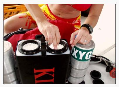
Wipe the top and inside edge of the canister once it has been filled. Also wipe the edges of the hose attachment connectors clean.
