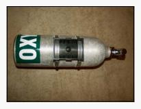
We have found that after a year or two of use, the tank mounting system can start to wear. If this happens the cylinders can pop out of the holder. First flip the mount on the cylinder. By doing this, you should get more life from the mount. Also, at some point, the lever may need to be replaced also. The lever will need to be replaced after a year or two of wear, or if it breaks.
