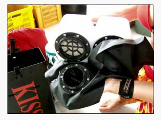
Lift the scrubber canister out of the counterlung case and remove the counterlungs. The lungs are removed by rotating them 1/4 turn counter-clockwise.
