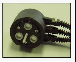
Attach the sensor assembly to the display pod, ensuring that the N7O-O34 O-ring on the sensor assembly is in place and lubricated. The assembly needs to be attached to the side of the pod which has a groove machined into it. Please see the photo to the right and to the bottom for groove placement. The flat edge of the sensor assembly needs to be positioned at the bottom side of the pod.
