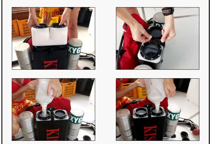
Once the canister has been replaced in the counterlung case and is secure, it is ready to be filled. Start by pouring scrubber into both sides of the canister.
