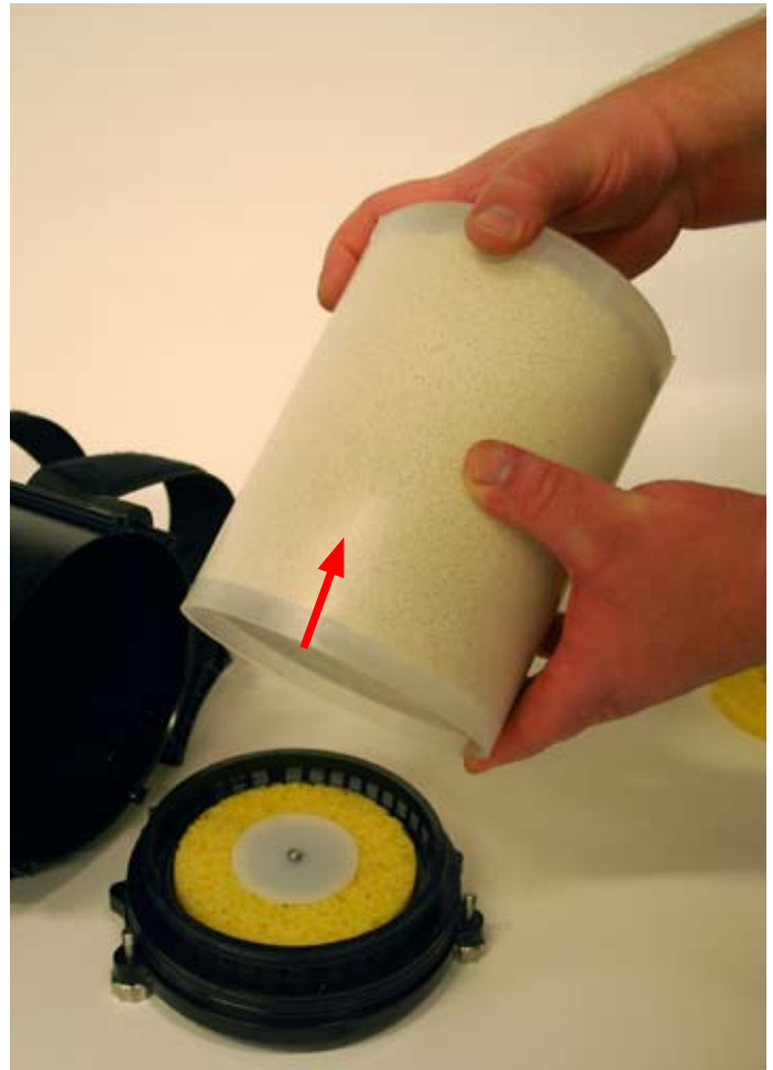
Figure 1-17. Remove the end plate.
