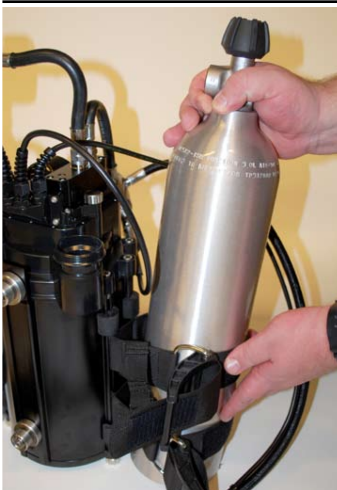
Figure 1-44. Insert the diluent cylinder into the two right cam straps.
