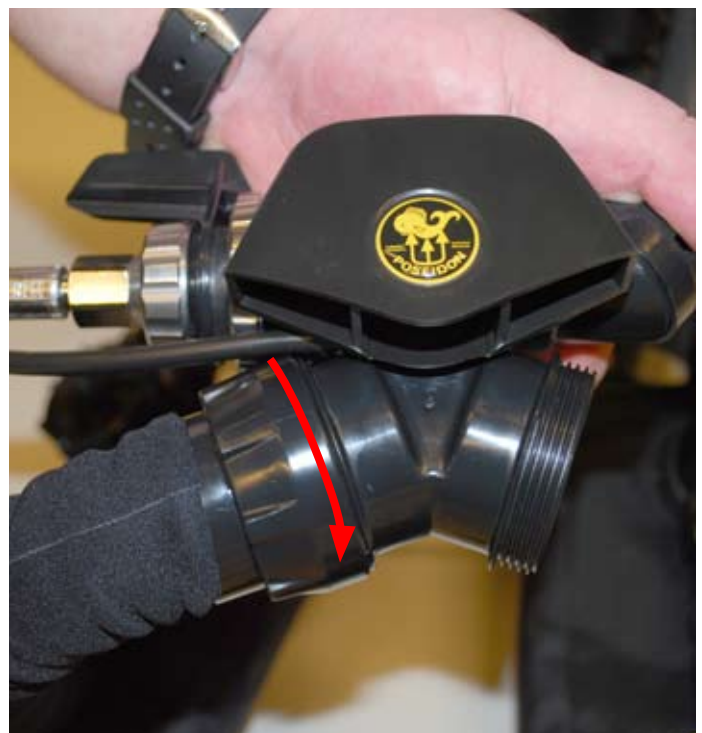
Figure 1-73. Tighten the hose nut on the downstream CC port threads. DO NOT use tools or over-tighten.
