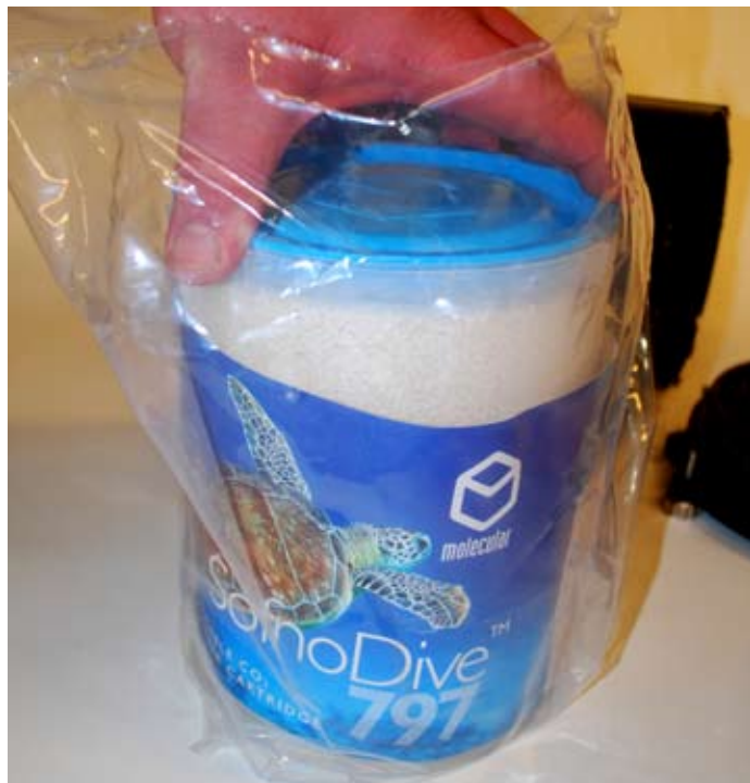
Figure 1-21. Opening the sealed SofnoDive 797 air-tight shipping envelope
