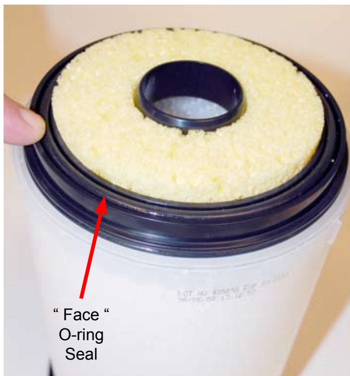
Figure 1-9. Typical “Face” type o-ring seal.
