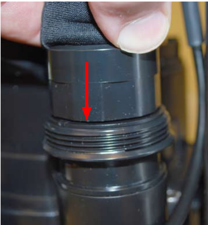
Figure 1-55. Push hose connector into receiver until outer flange is flush with start of threads.
