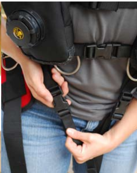
Figure 1-99. Attach the right counterlung retainer buckle and cinch it down.
