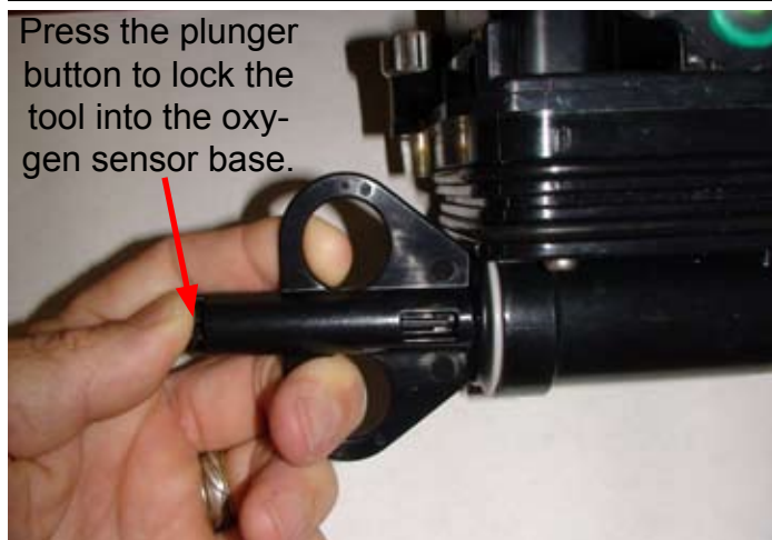
Figure 4-3. Press button to lock tool onto sensor base.
