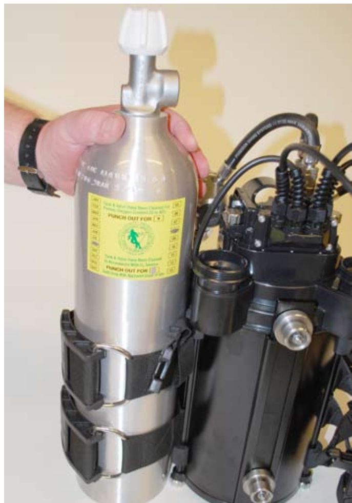
Figure 1-41. Follow the same threading, tightening, and latch procedure for the lower buckle and diluent cylinder.
