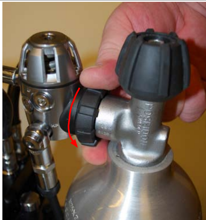
Figure 1-47. Hand tighten the diluent swivel nut.
