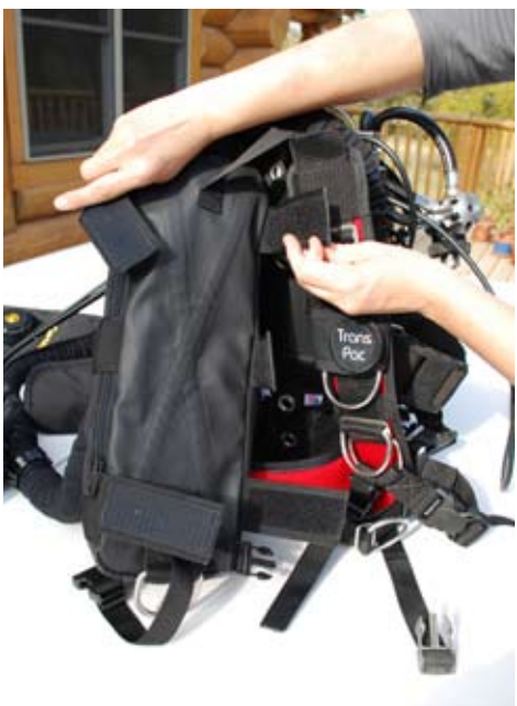
Figure 1-88. Open the 3 velcro straps on the back of the left counterlung.
