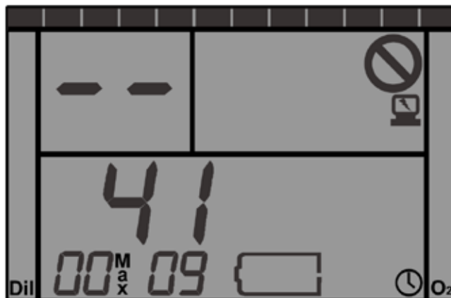
Figure 2-2. Initial displays during the first two seconds of Power-up, showing firmware version and serial number.
