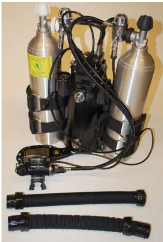
Figure 1-52. Lay out the two rear breathing hoses as shown.
