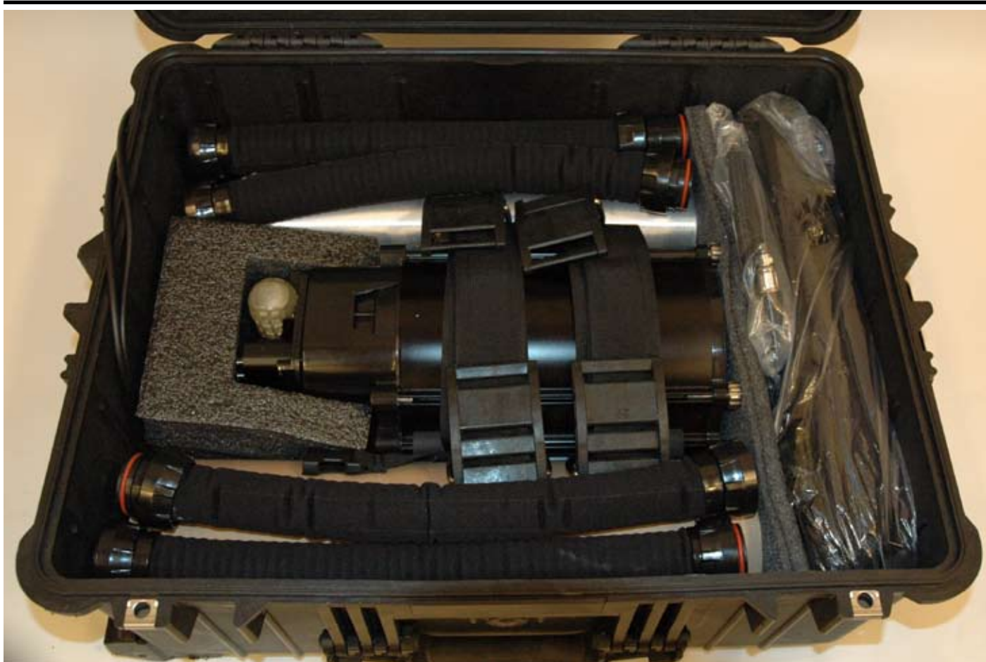
Figure 4-8. Lower layer of packing the case, with cylinders, hoses, counterlungs, backpack and electronics module.
