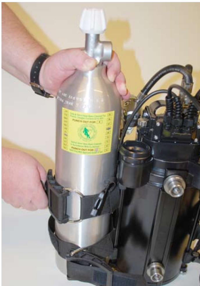
Figure 1-40. Latch the upper cam buckle.
