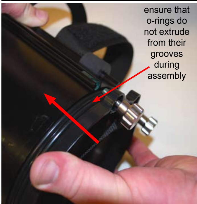
Figure 1-27. Final insertion of end cap into cartridge housing - Figure 1-28. Tighten the four hand nuts
