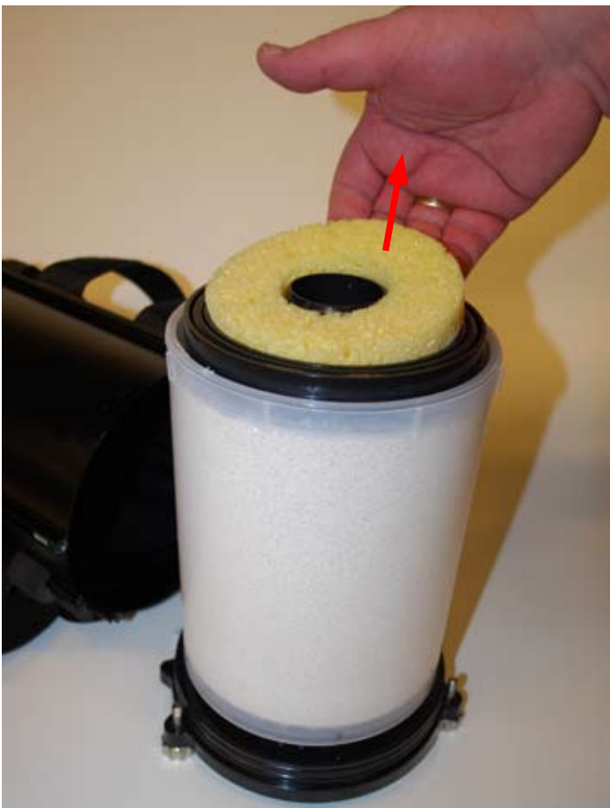
Figure 1-14. Lift and remove the upper sponge.
