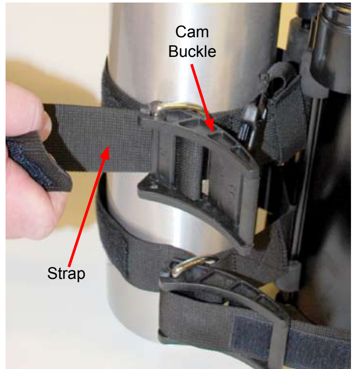
Figure 1-37. Pull the upper strap tight against the cylinder. Note the webbing path through the cam buckle.
