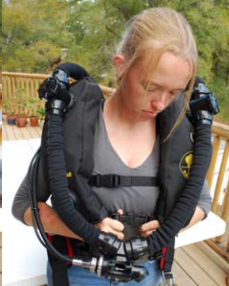
Figure 1-96. Attach the counterlung cross strap.
