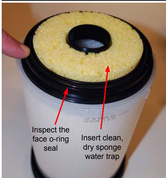
Figure 1-24. Insert cartridge top plate and sponge into the water trap, and inspect the face-seal o-ring.
