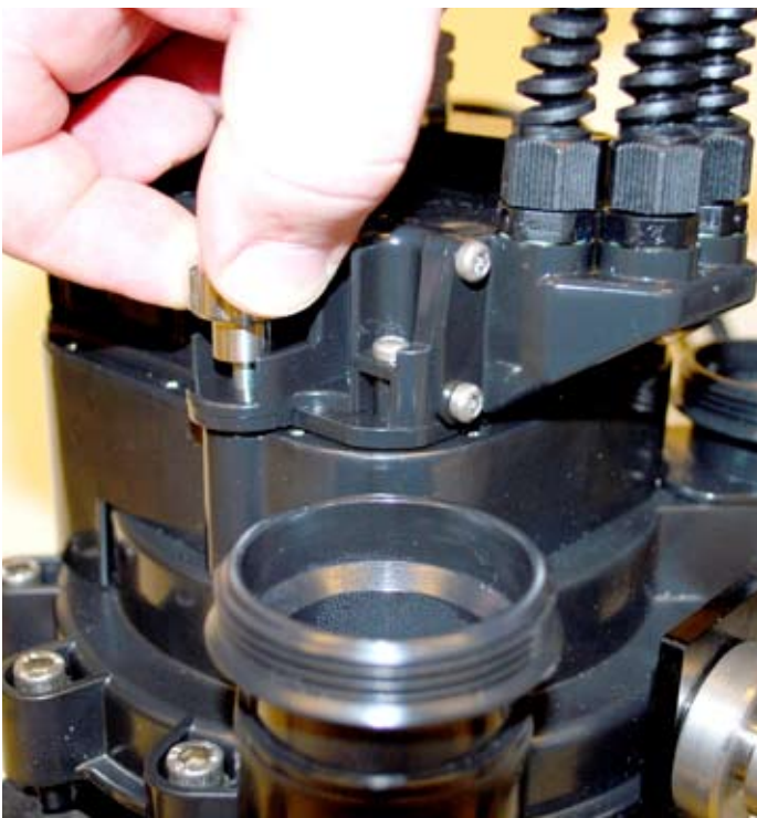
Figure 1-33. Firmly screw down the hand nut on the right side of the electronics housing (use NO tools)
